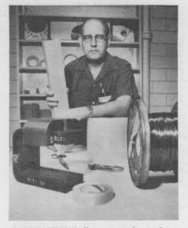
RAW MATERIALS all come together in Sandia's Transformer Shop and emerge as transformers, coils and other pieces of electrical gear. Typical materials assembled here and displayed by Henry Wellers include laminated transformer core, enamelled copper wire for windings, plastic sheeting for insulating windings, a square cardboard mandrel, and tools for handling materials.
